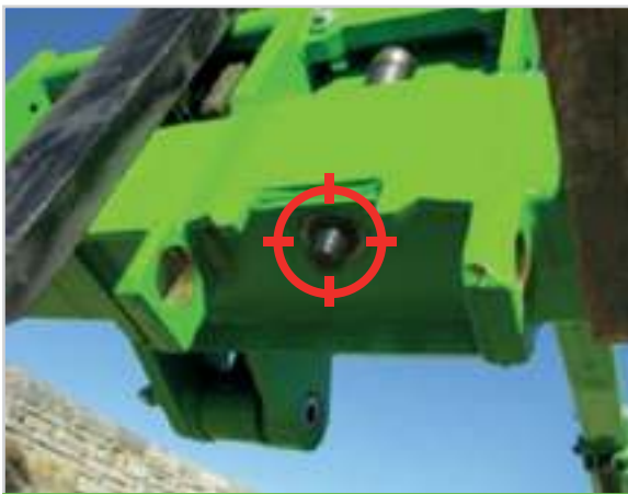
Tac-Lock: hydraulic attachment clamping system from the cab
