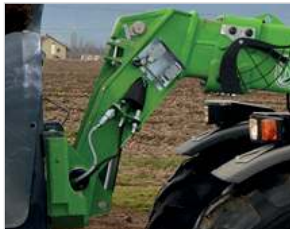
Pipes, power cables and auxiliary hydraulic are all located inside the boom
